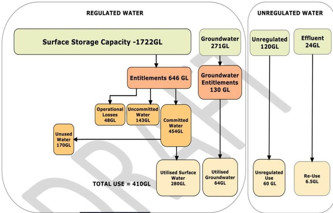
Figure A.2: Irrigation Water Use in WBB and Gross Value (extracted from paper)
